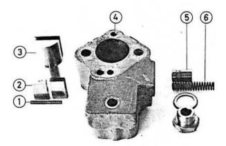
Fig. 40. Lubricating oil pump
