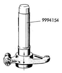
Fig. 18. Replacing a rocker arm bushing.
