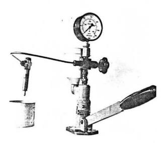
Fig. 52. Injector tester
