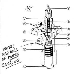
Fig. 48. Injection pump, Dl and MDl
