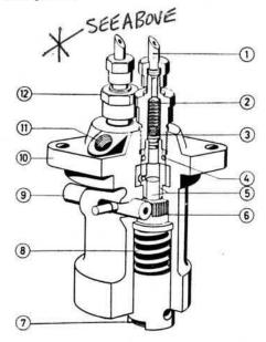
Fig. 49. Injection pump, D2 and MD2
