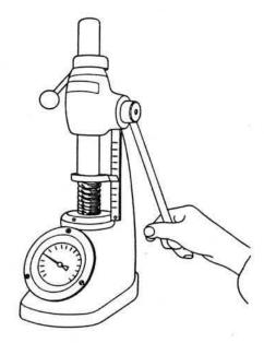
Fig. 16 Checking a valve spring.
