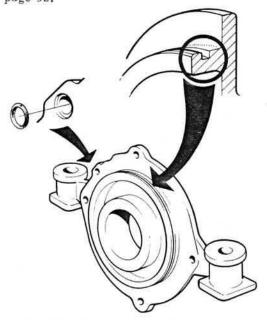
Fig. 35. Crankcase and bearing cover sealing.
