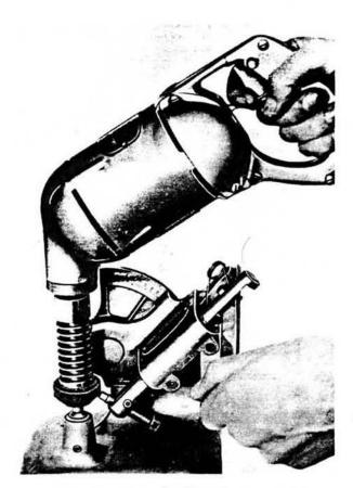
Fig. 13. Dressing the grinding stone.
