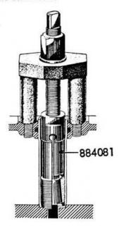
Fig 7. Removing the injector sleeve.
