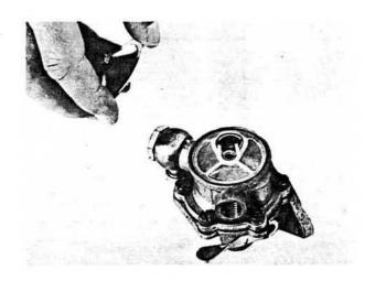
Fig. 64. Cleaning the strainer.
