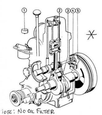
Fig. 38. Lubricating system, Dl and MDl
