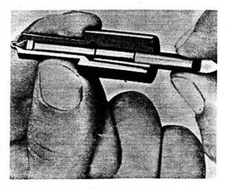
Fig. 57. Cleaning the nozzle seat
