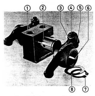
Fig. 17. Rocker arm mechanism
