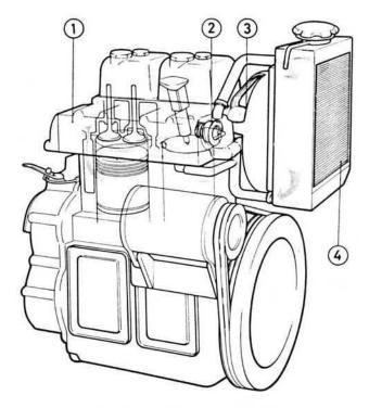
Fig. 67. Cooling system, D2
