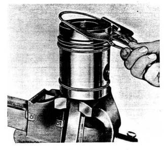
Fig. 25. Fitting the piston rings
