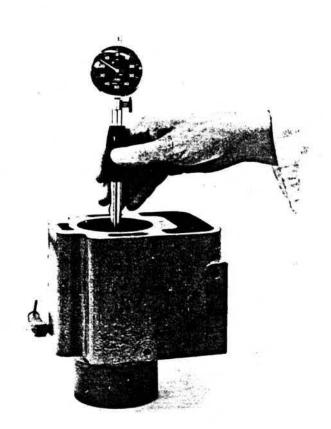
Fig. 21. Measuring cylinder bore wear.
