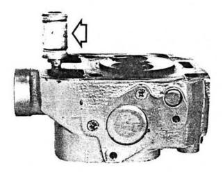
Fig. 41. Crankcase ventilation
