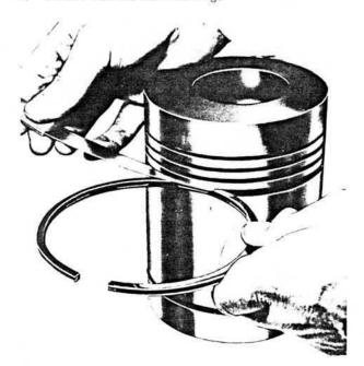
Fig. 24. Piston ring clearance in groove
