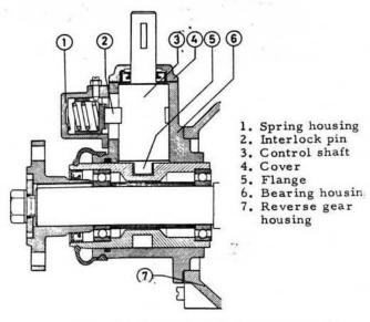
Fig. 71. Rear section of reverse gear
