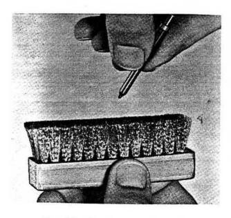
Fig. 54. Cleaning a nozzle needle
