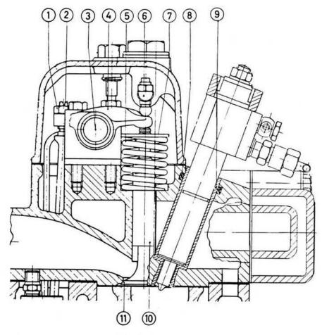
Fig 6. Cylinder head and valves
