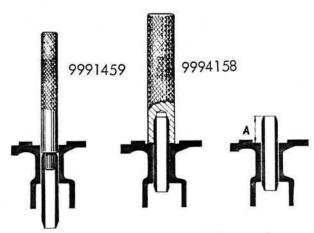
Fig. 12. Removing and fitting valve guides.
