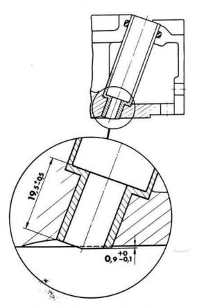
Fig. 10 Adjusting the sleeve
