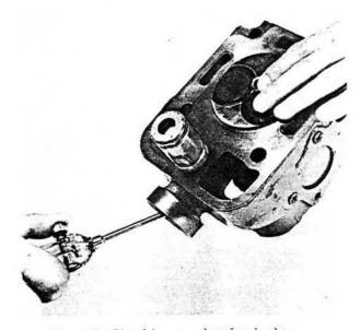
Fig. 15. Checking a valve for leakage.
