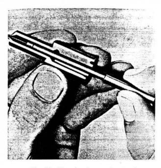
Fig. 56. Cleaning the nozzle chamber
