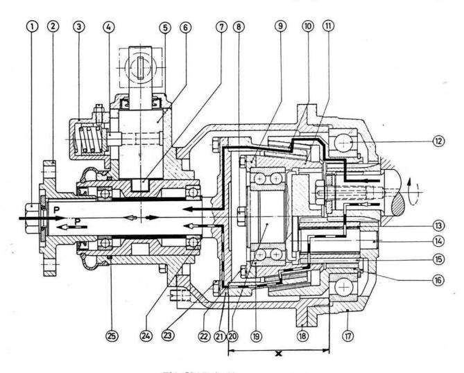
Fig. 70. Reduction - reverse gear
