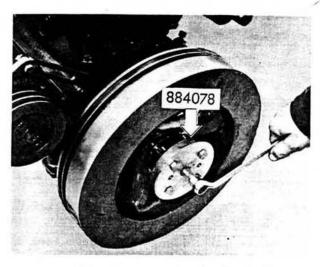
Fig. 37. Removing the flywheel.
