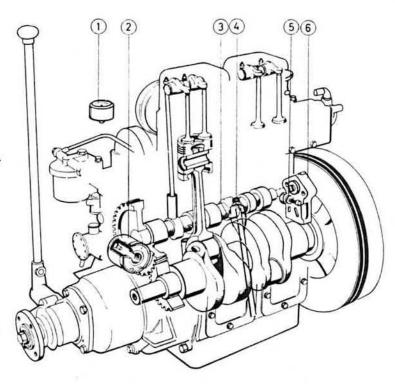
Fig. 39. Lubricating system, D2 and MD2
