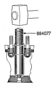
Fig 8. Pressing in the injector sleeve
