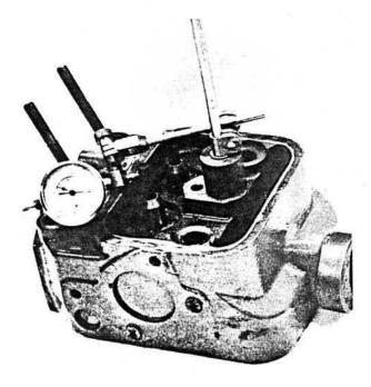
Fig. 11. Checking valve guide wear.
